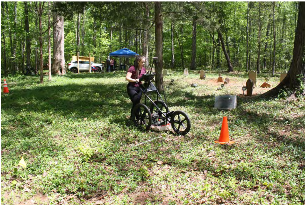
Figure 4.5: Cayla Cannon, RGA's Geophysical Specialist, conducting a ground-penetrating radar (GPR) survey at the Kiser-Huffstetler Cemetery in Lincolnton, North Carolina.
