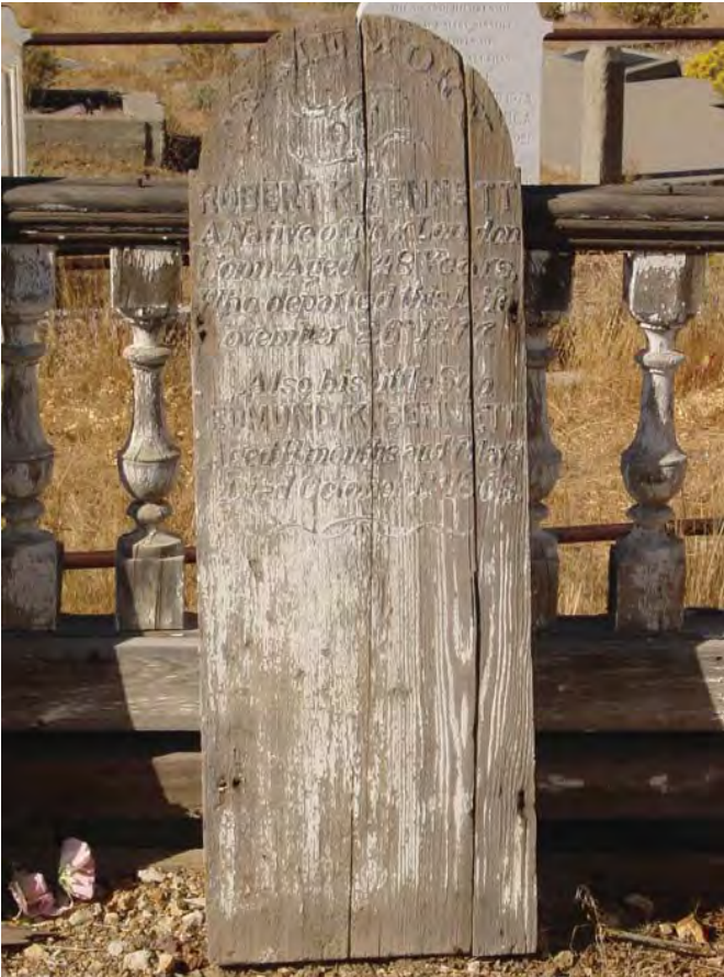
Figure 7. As shown by this 1877 marker in Silver Terrace Cemetery, Virginia City, NV, exposure to sunlight can damage wood grave markers, making the wood more susceptible to water damage and cracking. Photo: Jason Church.
