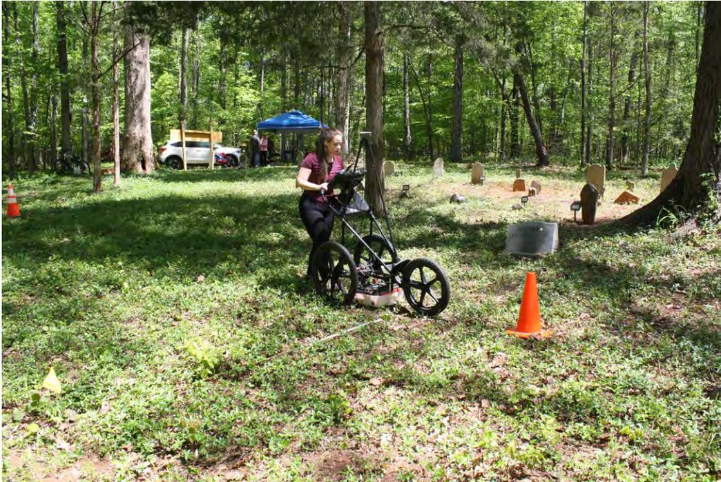
Figure 4.3: Cayla Cannon, RGA's Geophysical Specialist, conducting a ground-penetrating radar (GPR) survey at the Kiser-Huffstetler Cemetery in Lincolnton, North Carolina.
