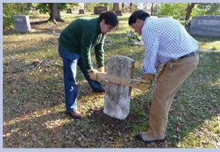
Figure E1. The simple wooden clamp system allows two people to safety lift a marble grave marker. Photo: Sarah Jackson.
