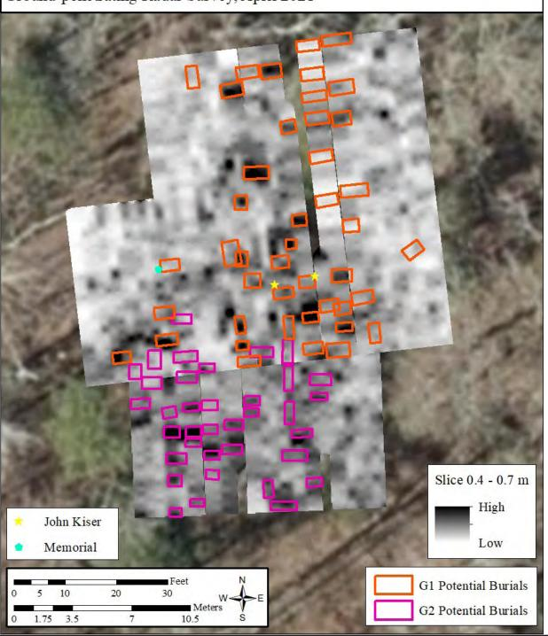
Figure 4.4: A total of 80 potential burials were identified through post-processing during the GPR survey of the Kister-Huffstetler Cemetery. This number includes 44 potential marked and 36 potential unmarked burial anomalies. This graphic shows potential burials in Grids 1 and 2 on a time slice map at 0.4 to 0.7 meters below the surface.
