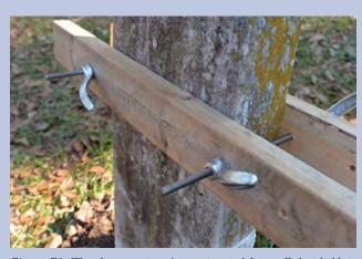
Figure E2. The clamp system is constructed from off-the-shelf wooden boards. Photo: Sarah Jackson.
