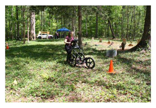
Figure 4.3: Cayla Cannon, RGA's Geophysical Archaeologist, conducting a ground-penetrating radar (GPR) survey at the Kiser-Huffstetler Cemetery in Lincolnton, North Carolina.
